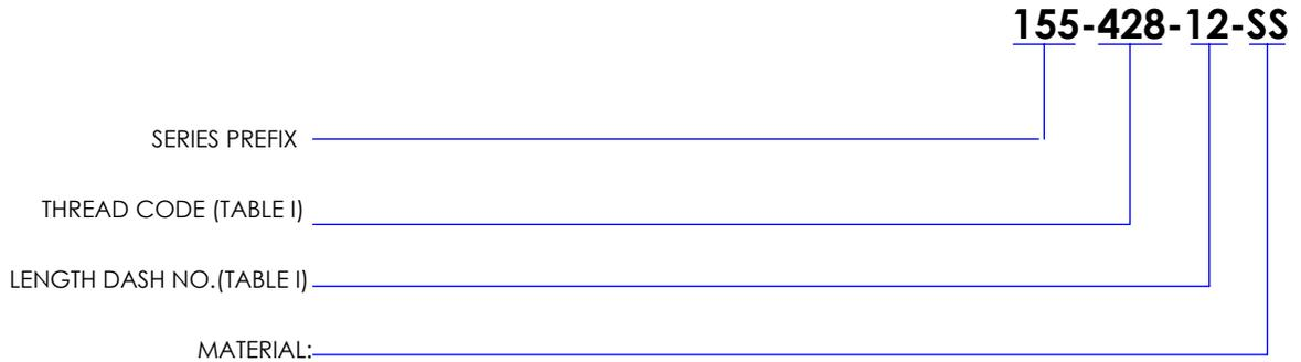
A= ALUMINUM(CHEM FILM FINISH)HOUSING & CAP WITH CARBON STEEL NUT (CADMIUM PLATED).
