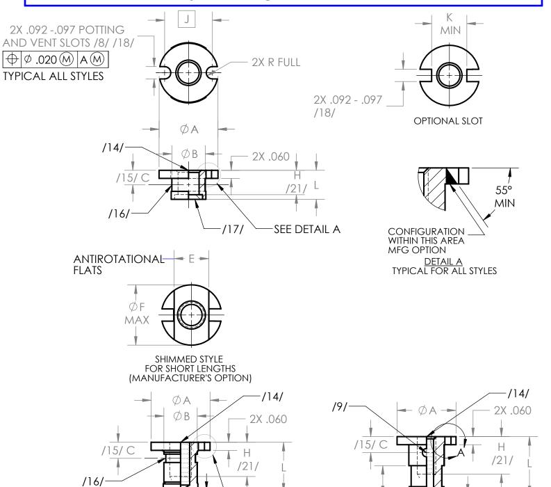
BLIND TAPPED STYLE FOR LONG LENGTHS ALL STEEL AND CRES SELF-LOCKING AND NONSELF-LOCKING OR NONSELF-LOCKING ALUMINUM STYLE.
